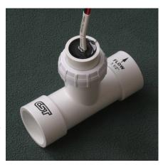
The flow sensor housing, held in place with a retaining nut, contains the detection circuitry and carries the unique four-bladed impeller on a transverse axle. The housing and mounting tee are custom molded to form an integrated measurement chamber resulting in highly accurate, repeatable flow measurements through a wide range of velocities. The axle and impeller along with the sealing o-ring are replaceable in the field.
